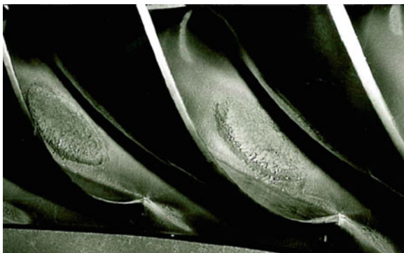
Fig. 2.17 Cavitation erosion caused by inter blade vortex
