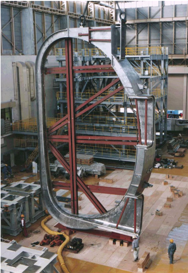
Fig. 2.12 One segment of the ITER vacuum chamber model. Note the person at the bottom . Courtesy of ITER Organization
