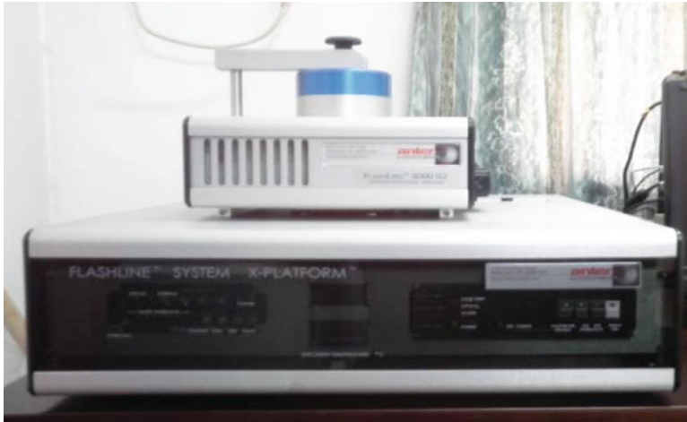
Fig. 2.2 Flash method equipment for measuring thermal conductivity
