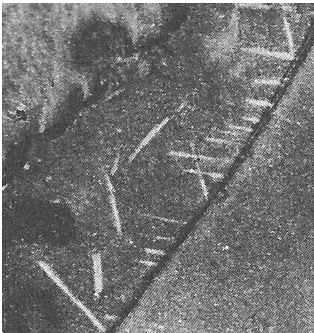
Fig. 2.8 A fringe of rutile needles at the alumina-bond contact. Reflected light, \times 250 magnification (Courtesy of Professor Givi Bockuchava)
