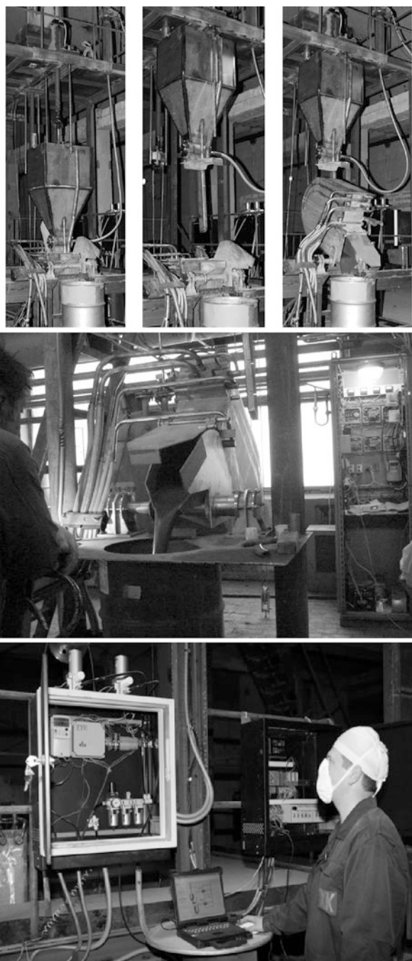
Fig. 2.6 Cementation pilot facility with pulse mixer
