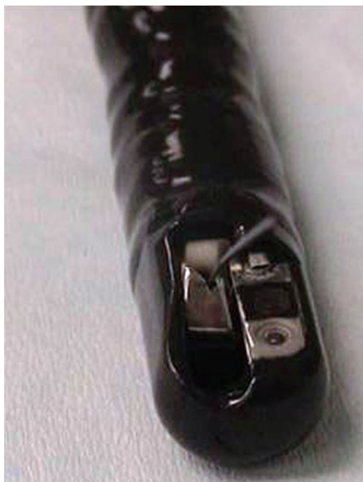
Fig. 2.12 The V-scope system with a small notch created on the elevator mechanism
