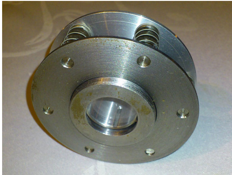
Fig. 2.11 Experimental device for the compression of samples according to Fig. 2.10, for use in interferometer for recording deformation. Samples placed on round glass surface in the middle, to be covered by interferometer mirror
