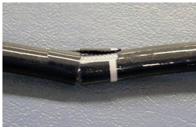
Fig. 2.19 Wearing and erosion through autoclaving of normal endoscopes
