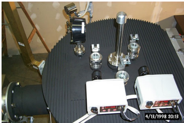
Fig. 2.10 This is an example of a process and over temperature pyrometer being used to control temperature. This configuration is for a microwave caster, but the equipment and setup are the same for microwave, VIM, and VAR
