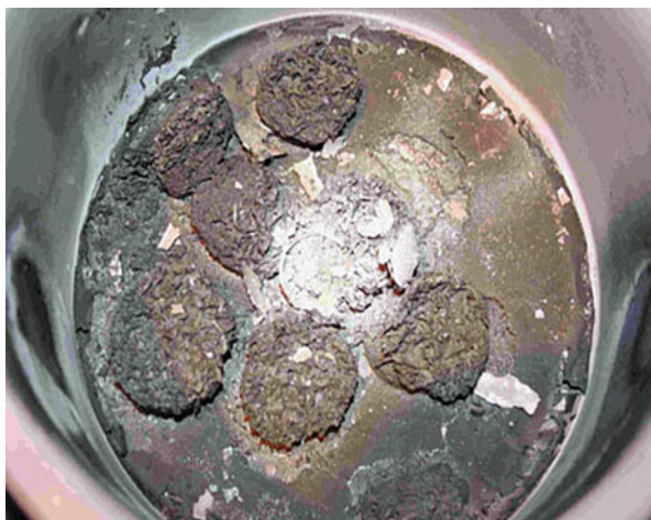
Fig. 2.18 The solid oxide shells often referred to as ghosts , which are left in the crucible when the uranium is melted and poured into the mold
