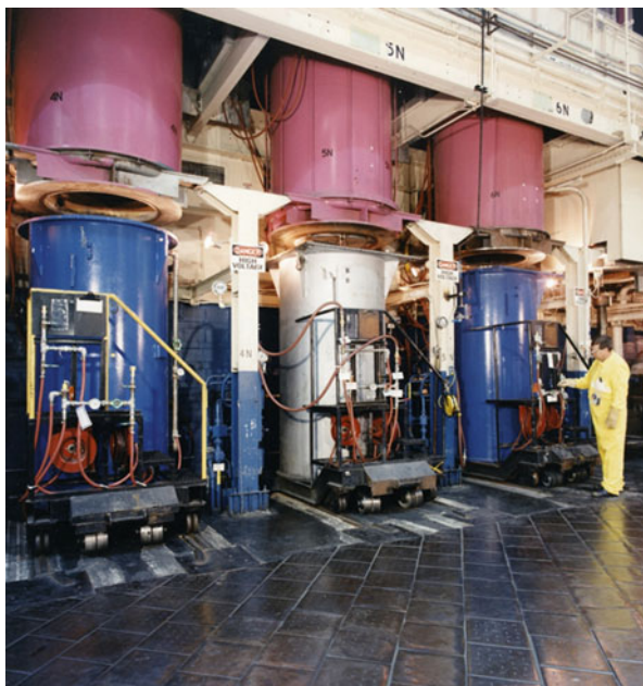
Fig. 2.1 Example of a large bottom-loading vacuum induction casting line. Stack loading and unloading occur on this first floor, and the furnace is operated from the second floor
