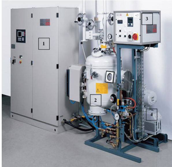
Fig. 2.3 VIM caster showing (1) power supply, (2) chamber (with crucible and mold inside), (3) control panel, and (4) vacuum system
