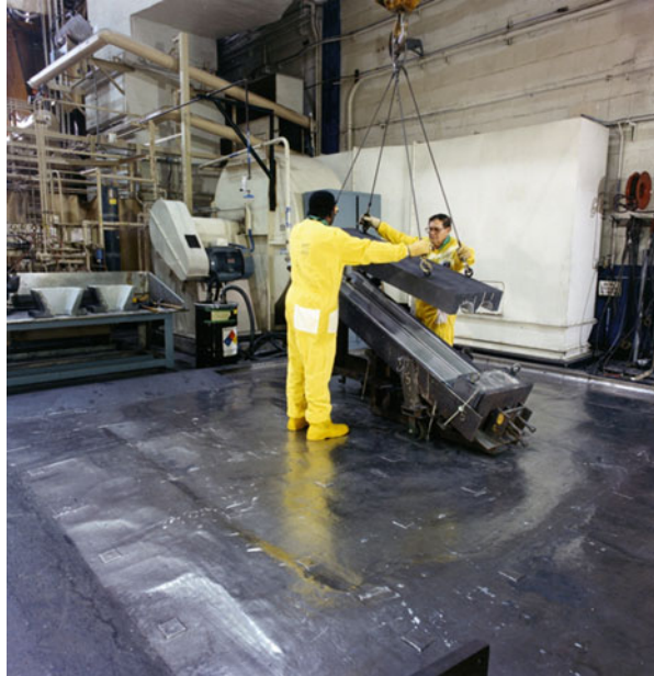
Fig. 2.6 Example of mold that has been coated to prevent contamination of the metal by the mold and to facilitate releasing the casting from the mold
