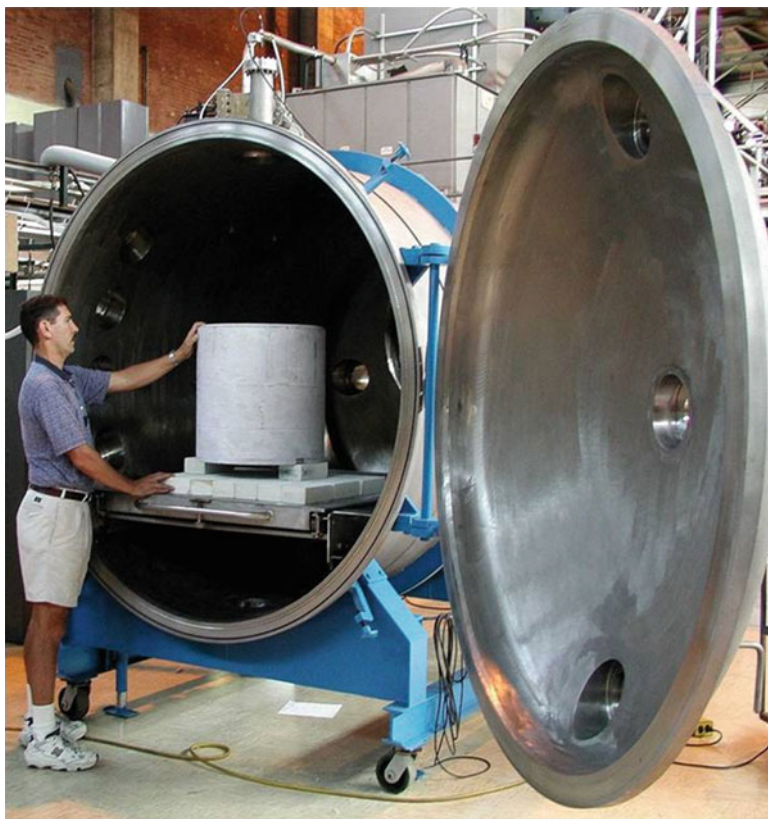
Fig. 2.16 Large front loading microwave chamber for casting high-temperature reactive metals
