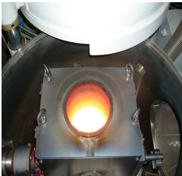
Fig. 2.5 This is the coil that was shown in Fig. 2.4 installed in a system. The molten metal in the crucible is a surrogate for this demonstration
