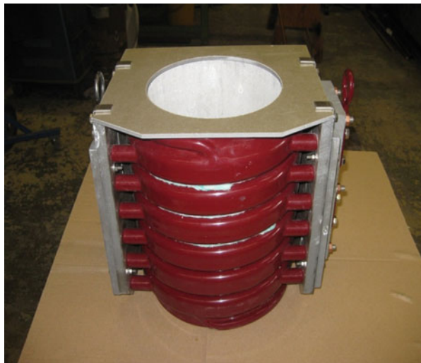
Fig. 2.4 This is a VIM coil used in a tilt pour system for casting of reactive metals
