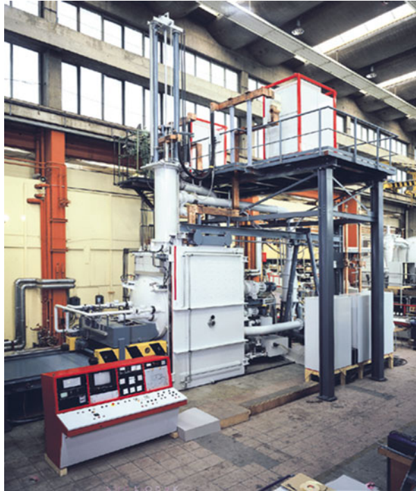
Fig. 2.9 VAR system showing major components for operation
