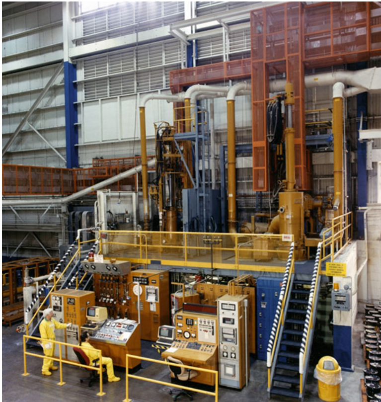
Fig. 2.7 Example of large VAR unit, which makes high-purity alloys for further processing
