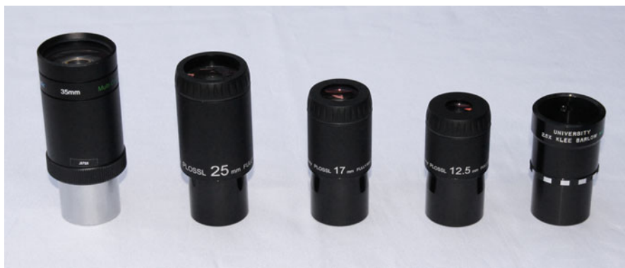
Fig. 2.16 Example of how strategically using a Barlow allows almost no focal length overlap. No Barlow—35 mm, 25 mm, 17 mm, and 12.5 mm. With 2.8× Barlow—12.5 mm, 8.9 mm, 6.1 mm, and 4.5 mm (Image by the author)
