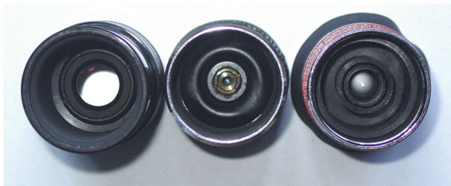
Fig. 2.7 Inside of barrels: well blackened ( left ), bare metal parts ( center ), plastic parts ( right ) (Image by the author)
