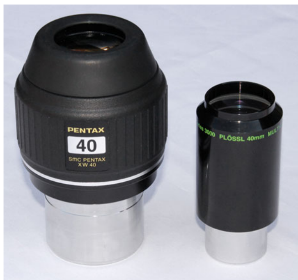
Fig. 2.8 Examples of size and weight variations of eyepieces. 40 mm Pentax XW ( left ) vs. 40 mm Meade 3000 Plössl ( right ) (Image by the author)
