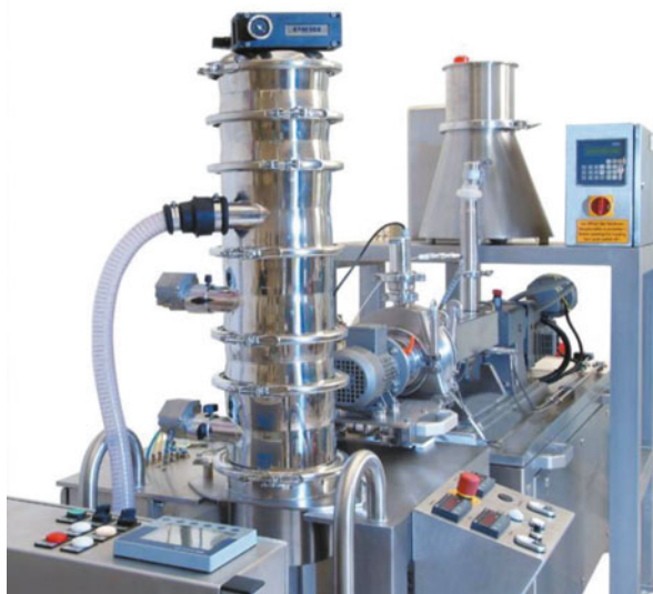
Fig. 2.26 Micro-pelletizer attached to TSE
