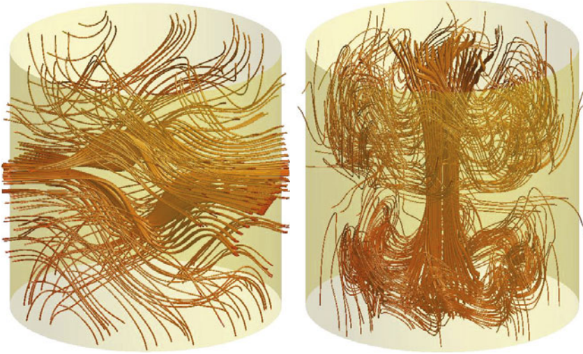
FIGURE 7. Geometry of the dynamo mode obtained by kinematic numerical simulations: (Left) an equatorial dipole is generated by the mean flow alone. (Right) When a non axisymmetric velocity component is taken into account, an axial dipole is generated. From [32] with permission from © 2009 IOP Publishing.
