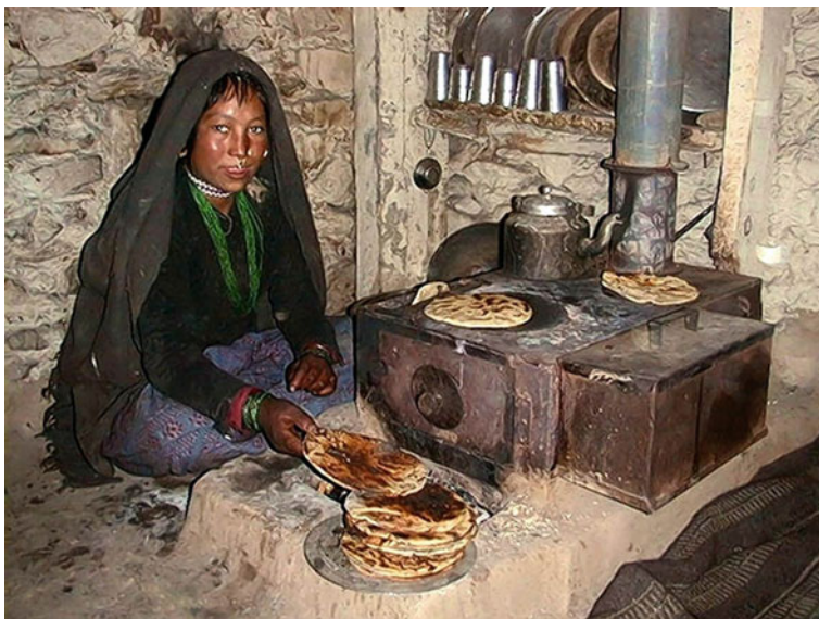
Fig. 2.14 The Smokeless Metal Stove (SMS), designed by the author in 1998. Up to 2011 an estimated 25,000 homes (through RIDS-Nepal, the government subsidy program and other NGOs) in the remote districts of Nepal have had this SMS now installed. It cooks the traditional food all at one time, uses ~40 % less firewood, provides appropriate room heating and 9 liters of hot water for drinking the local “butter tea” as well as facilitating an improvement in personal hygiene. This is called “contextualised” technology, with people, their culture and way of living in the centre and technology developed to suit them in their context
