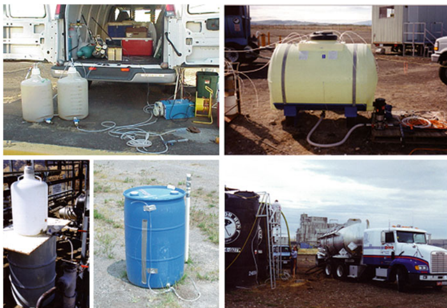
Fig. 2.1 Field push-pull test photographs showing various methods used to prepare and inject test solutions. Clockwise from upper left : separately prepared tests solutions in 50 L plastic carboys being combined and injected into a well using a peristaltic pump; 500 L test solution prepared in plastic tank; 240,000 L test solution being transferred from tanker truck to large plastic tank prior to injection; test solution in 200 L plastic drum being injected into monitoring well using a siphon; 50 L test solution in plastic carboy being injected into monitoring well by gravity drainage
