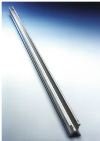
Fig. 2.22 The old international prototype of the meter: the famous platinum-iridium stick that defined the meter until 1960. Today the meter is defined by the speed of light in vacuum
