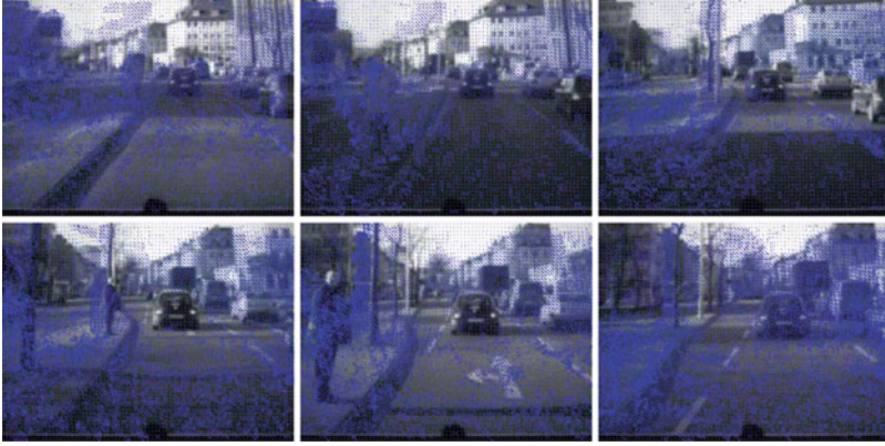
Fig. 1 On a traffic scene plotted motion vectors indicate regions, where a local flow estimator achieves reliable results. For significantly large regions the velocity can not be computed
