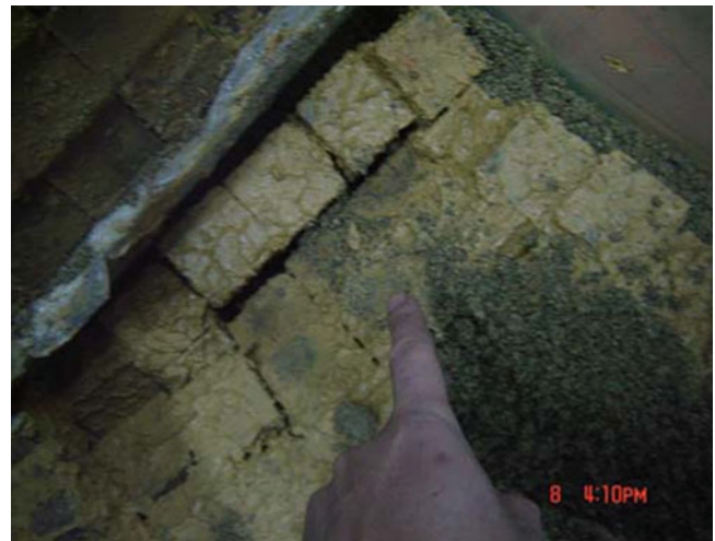
Picture 5 Polished surface and scrapes cinch marks clearly shown on the top slickenside
