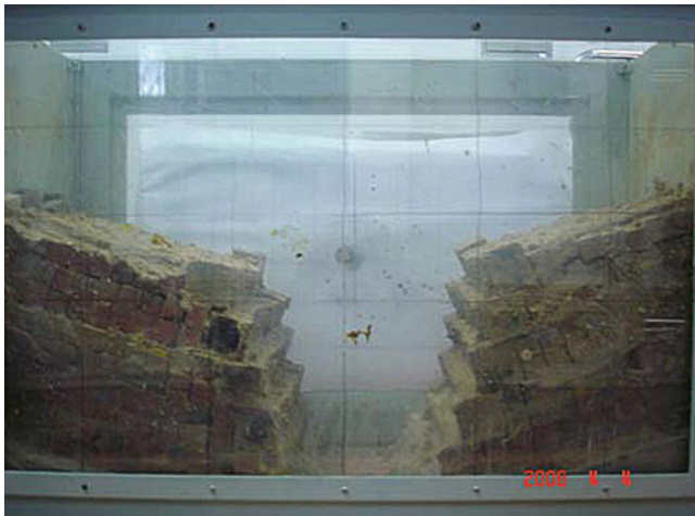
Picture 2 Model of slop dip toward excavation
