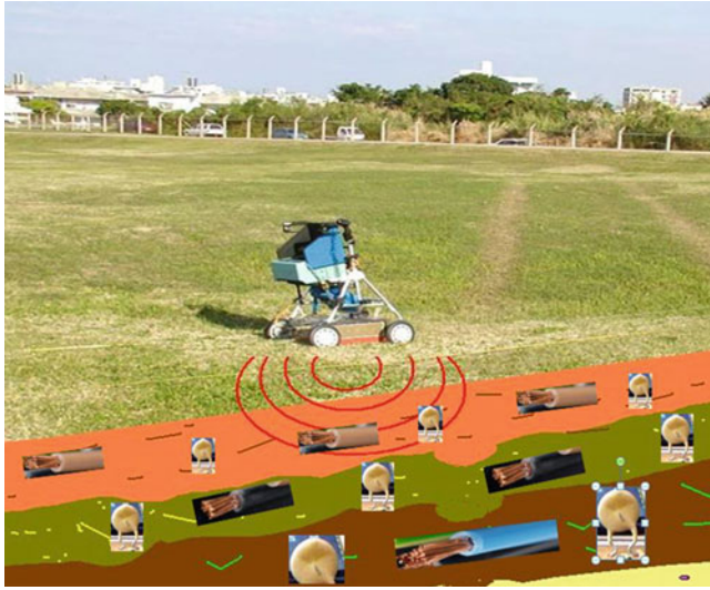
Fig. 2.1 A schematic diagram indicating an idealized ground which is composed of varying dielectric material and of wires having varying conductivity
