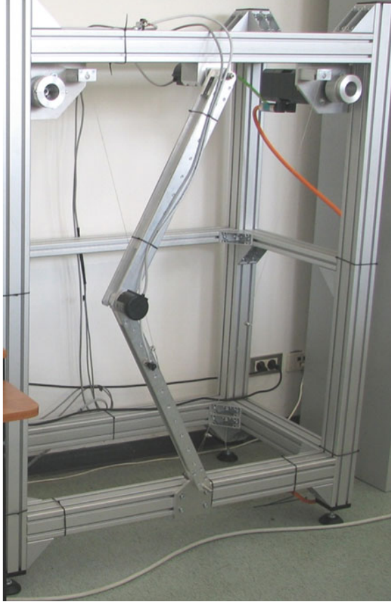
Fig. 2 Prototype of the planar CDDR
