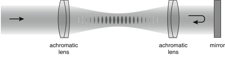
Fig. 2.5 An optical standing wave formed by retroreflection of a Gaussian laser beam creates a one-dimensional optical lattice potential. Generally, the electric field amplitude of the returning beam is reduced by a factor, which we call the effective reflection coefficient \rho
