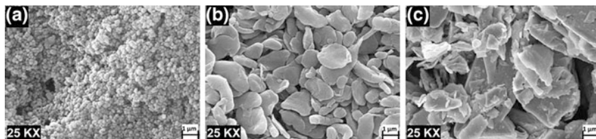
Fig. 3 FESEM micrographs of selected PTFE particles [19, 20]
