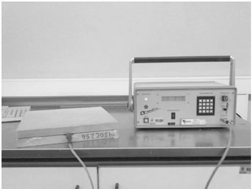
Fig. 2.3 Thermal shock method for determination of thermal conductivity of moist materials
