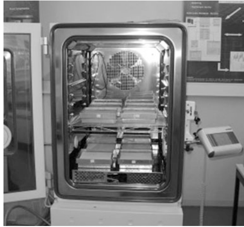
Fig. 2.6 Cups inside a climatic chamber
