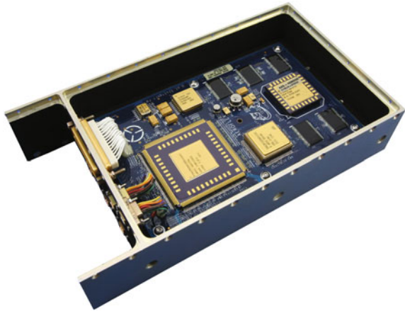
Fig. 2.1 OBC processor-board flight model in the mounting frame. © Aeroflex Inc./IRS, Uni Stuttgart
