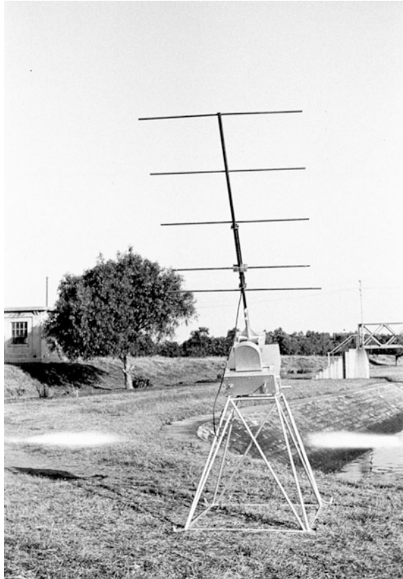
Fig. 2.14 Simple 65 MHz Yagi antenna used for routine solar radio astronomy monitoring. The antenna has an equatorial mount that enables continuous observations during daytime. The declination was set manually for each day. The antenna was located at the Potts Hill Reservoir (Chap. 10) of the Radiophysics Laboratory (RPL) of the CSIRO near Sydney Australia. The Yagi antenna was invented by Uda and Yagi in 1926 in Japan (CSIRO Radio Astronomy Image Archive B1465-1 from 26 July 1948)
