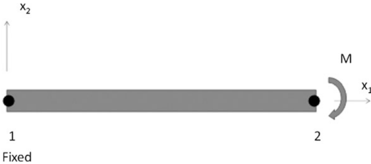
Fig. 2.2 Cantilever under constant moment modeled with one 4-node element: shear locking
