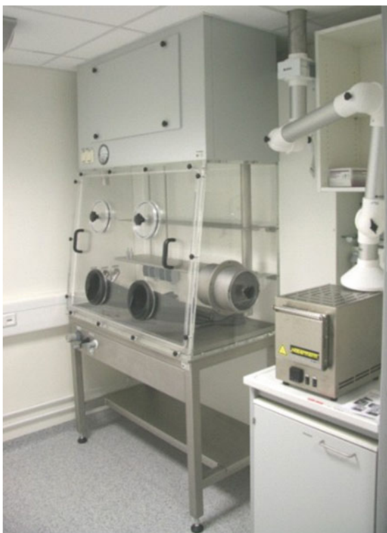
Fig. 2.12 Containment for the processing of radioactive substances in the nonpharmaceutical field (Source Isotope Technologies Dresden GmbH)
