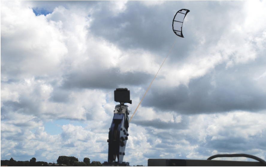
Fig. 2.1 A remote-controlled 25\text{m}^2 Leading Edge Inflatable (LEI) tube kite flying crosswind while pulling a 4mm cable with a force of 3kN from the ground station swivel, generating a traction power of 15kW [8]
