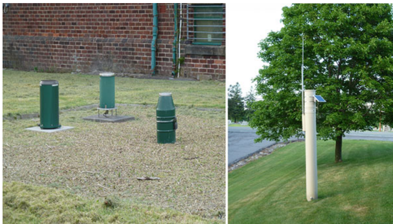
Fig. 2.2 Examples of raingauges at a weather station in the UK ( left ) and an IFLOWS installation in the USA ( right ). Integrated Flood Observing and Warning (IFLOWS) systems are widely used in flood warning systems in the eastern USA (e.g. see Box 6.1) and have similar origins to the ALERT protocol discussed in Chap. 3; here, the gauge is situated at the top of the structure, which also houses a data logger and telemetry equipment
