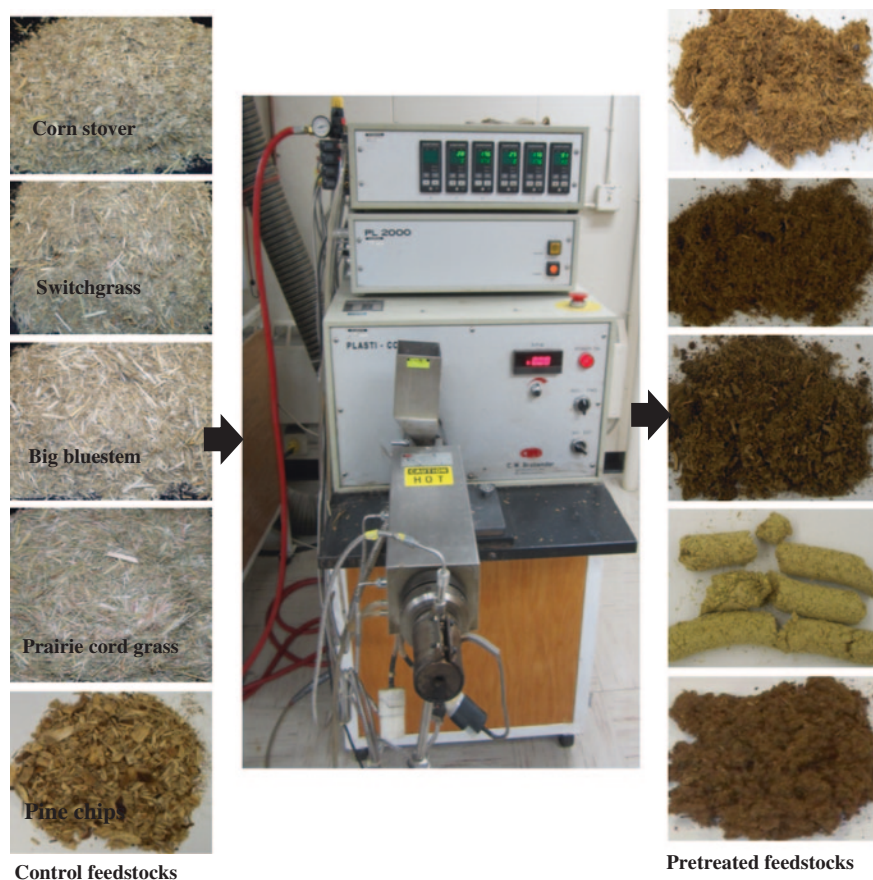
Fig. 2.6 Feedstocks pretreated in a single screw extruder
