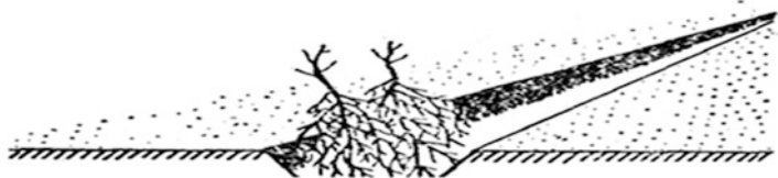
Fig. 2.20 Installation of materials in furrows
