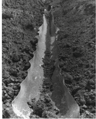
Fig. 2.3 Failure case of a gas pipeline with dynamic crack growth
