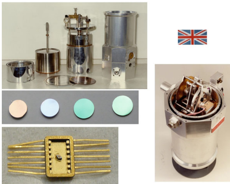
Fig. 2.3 Photometer cryostat with components
