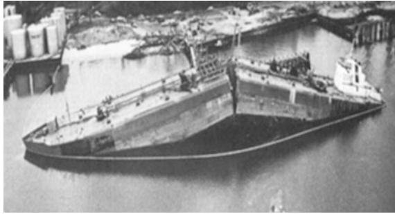
Fig. 2.13 Fracture of an oil tanker
