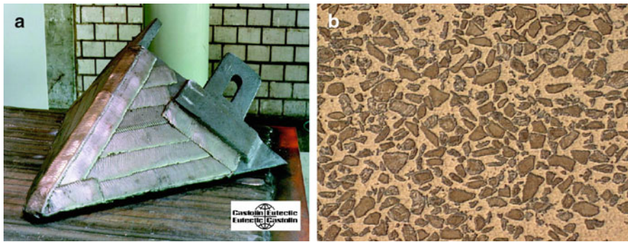
Fig. 2.16 (a) PTA-coated tooth of excavator with Ni base coating + WC (25 kg/h) and (b) cross section of the coating (courtesy of Castolin)
