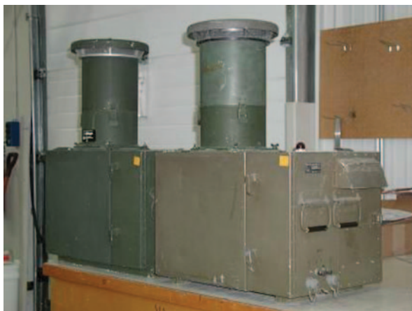
Fig. 2.3 XM19 ( left ), the detector and XM2 ( right ) the sample collector were designed to work electrically linked together. When the detector triggered an alarm from analysis of a biological aerosol presence, a signal was sent to the XM2 to initiate the collection of liquid samples. Note the provision of handles for mobility. In practice, hand carrying each unit was a two man effort
