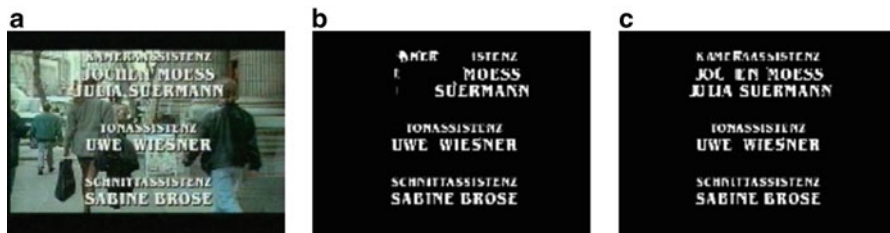
Fig. 2.16 Examples of the benefits of motion analysis for video text extraction: (a) original video frame, (b) text detection from a single video frame, and (c) better text detection for the same frame but using temporal redundancy for recovering lost characters [35]
