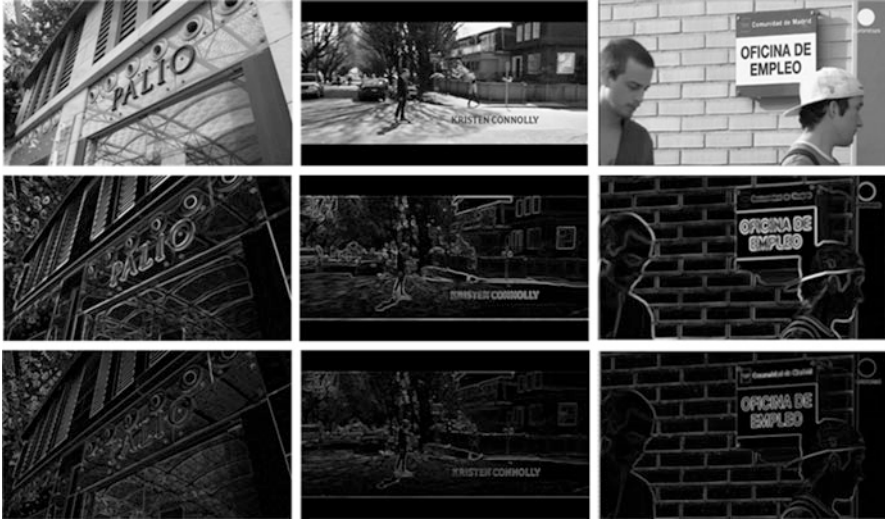
Fig. 2.12 Edge detection examples with the Canny operator on the second row and Sobel operator on the last row
