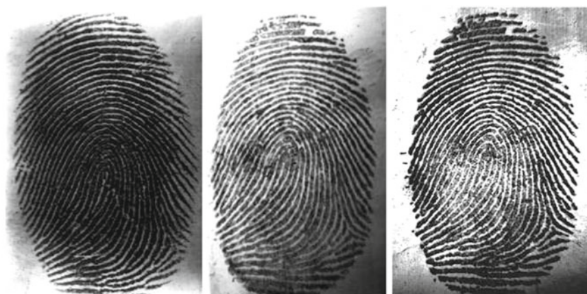
Genuine mark left by a finger on a glass plate visualized optically using co-axial episcopy
