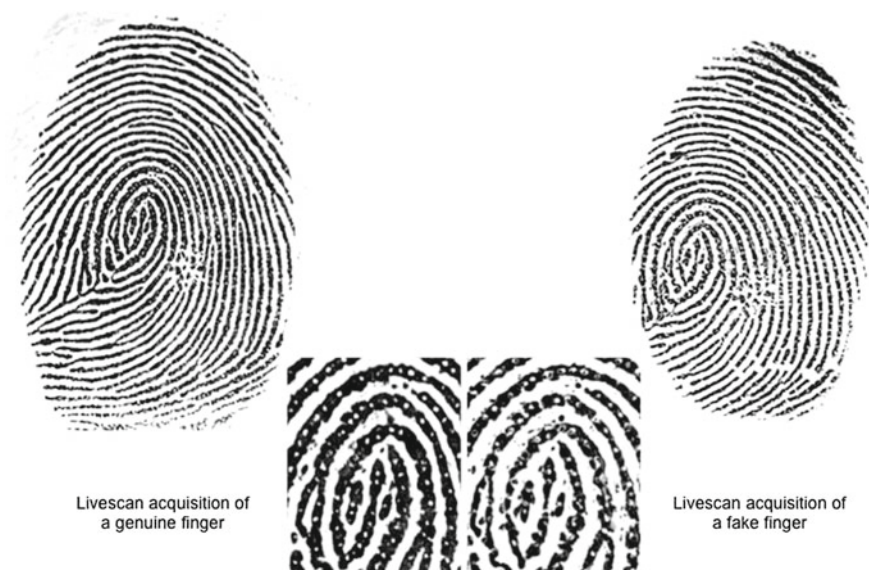
Fig. 2.6 Comparison between a genuine and a forged finger acquired on an optical livescan device. The forgery has been prepared using a double casting technique with the cooperation of the donor, the first mould is made in a thermoplastic (UtilePlast, Pascal Rosier, France), the second is a silicon molding paste (Siligum, Gédéon, France)
