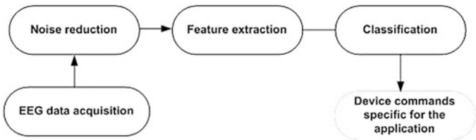
Fig. 2.2 EEG data processing for a BCI
