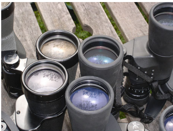
Fig. 2.21 Optical coatings. Clockwise from top left: single-layer coated, broadband multi-coated, multi-coated, uncoated
