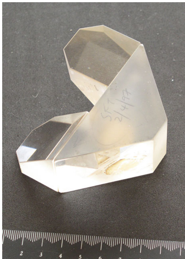
Fig. 2.6 Abbé erecting system, also known as a Porro type-2 prism
