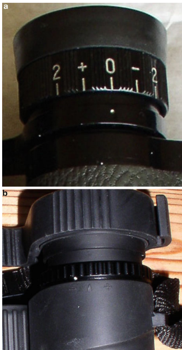
Fig. 2.29 Right eyepiece diopter adjustment. (a) Porro prism. (b) Roof prism
