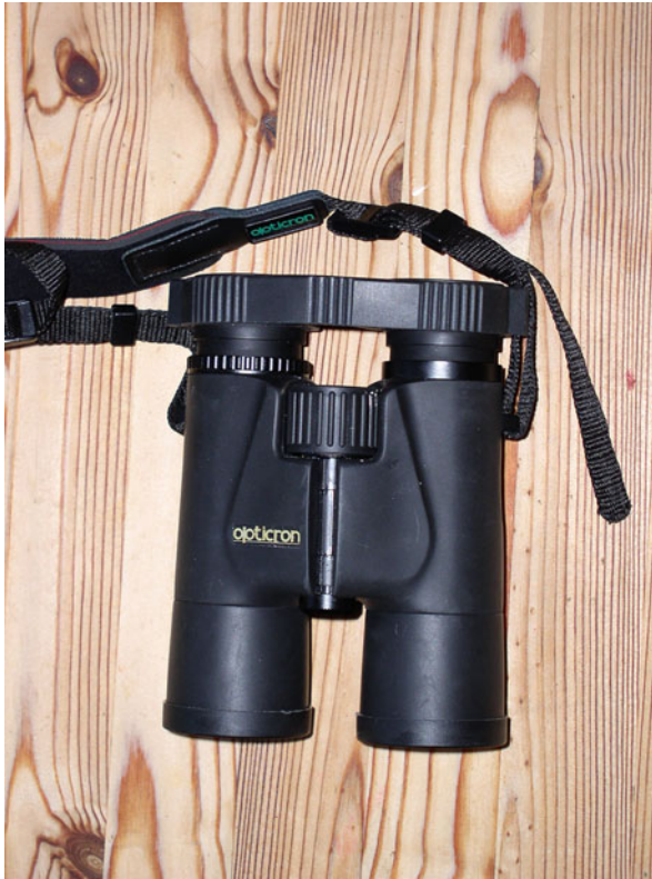
Fig. 2.31 Roof-prism center focus
