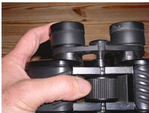
Fig. 2.30 The bridge rocks on this center-focus Porro-prism binocular
