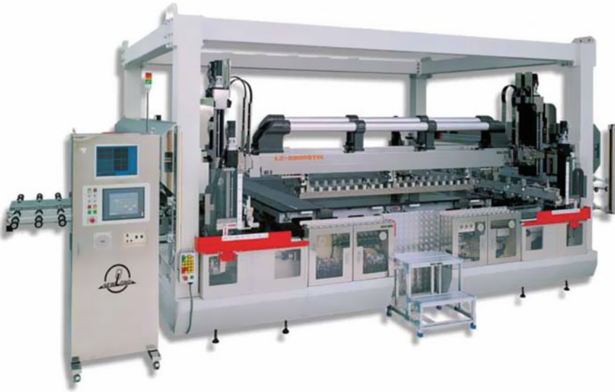
Fig. 2.10 Screen printer for large-scale PDP panel manufacturing (Courtesy of Newlong Machine Works, Tokyo, Japan)
