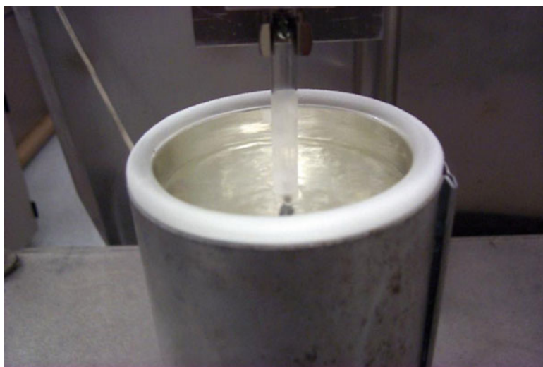
Fig. 4 Sample cooled in liquid nitrogen bath
