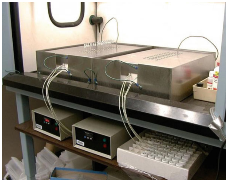
Fig. 2 Heating block used for heating samples
