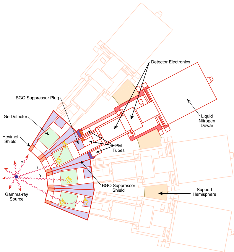
Fig. 2.8 Schematic of a Gammasphere detector module
