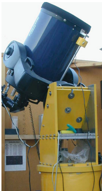
Fig. 2.2 Permanent pier and 12" LX-200 GPS telescope
