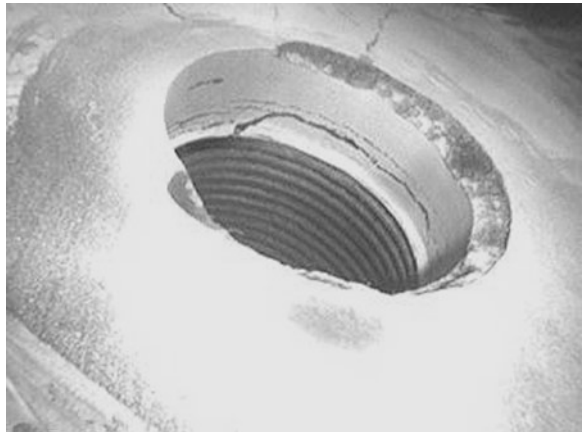
Fig. 2.21 Application of liquid penetrant to threaded bore
