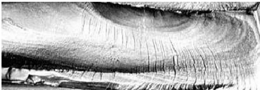
Fig. 2.13 Fatigue crack grown from the upper surface
