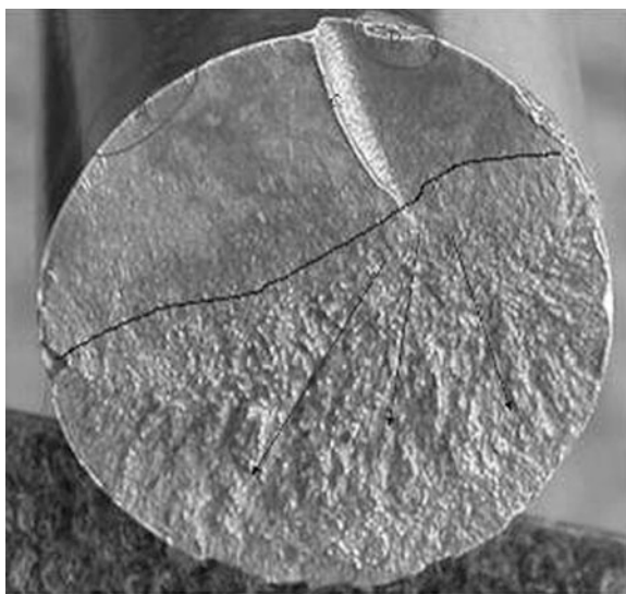
Fig. 2.16 Initiation sites separated by a ratchet mark
