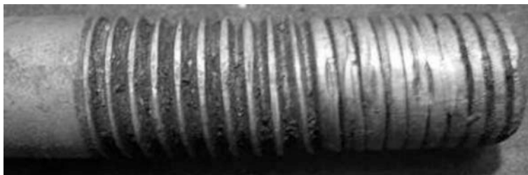
Fig. 2.C4 Worn out threads
