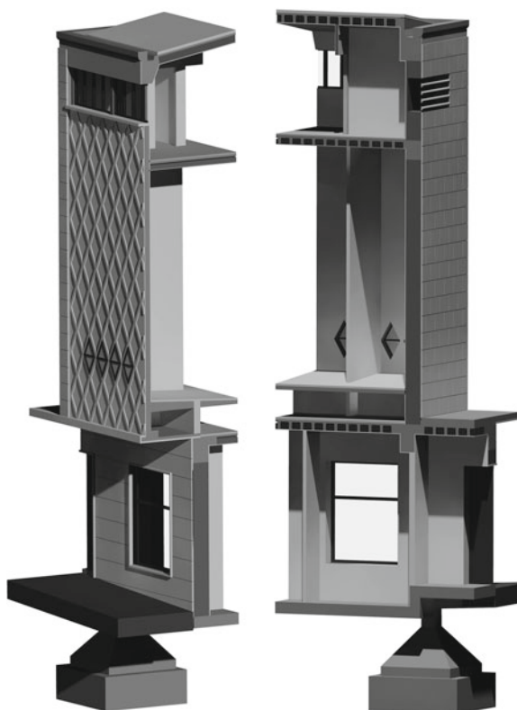
Fig. 14 Cinema Massimo in L'Aquila. Isometric render with detail's representation of the constructive system
