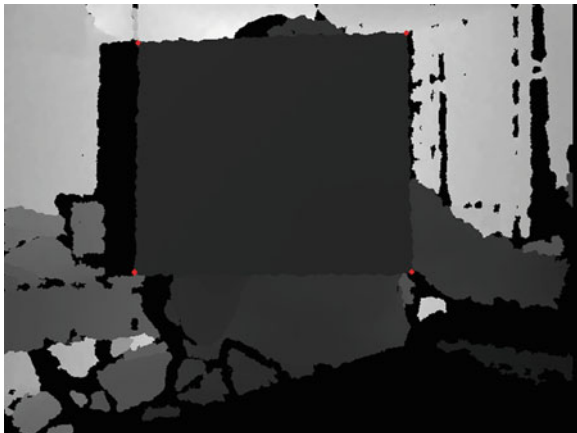
Fig. 6 The depth image consists of a chessboard with manually detected corners shown as red points
