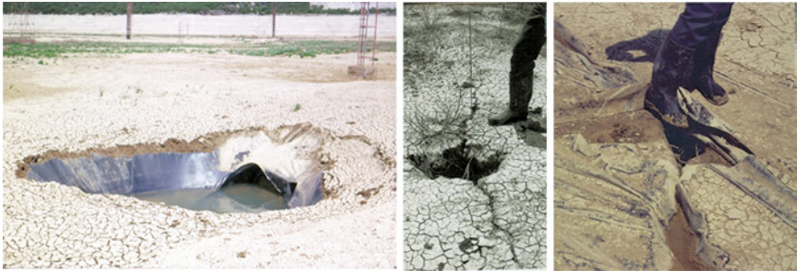
Fig. 19 Reservoir bottom (Hutovo, Herzegovina). Collapse and cracks beneath the geomembrane
