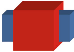
Fig. 1.18 Sketch of a stretching under the effect of the diagonal components of the strain tensor
