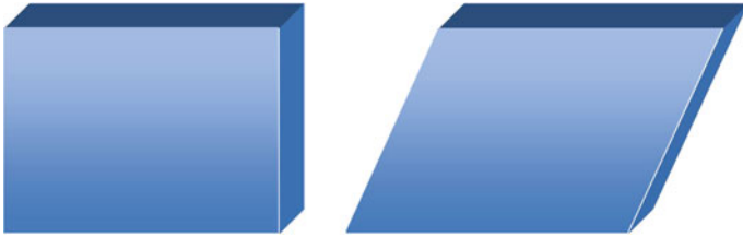
Fig. 1.19 Sketch of a shear ( right ) acting on an unstrained sample ( left ) under the effect of the off-diagonal components of the strain tensor
