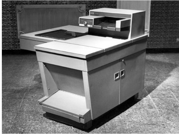
Fig. 2.1 Xerox 914 the first modern photocopier (1959)
