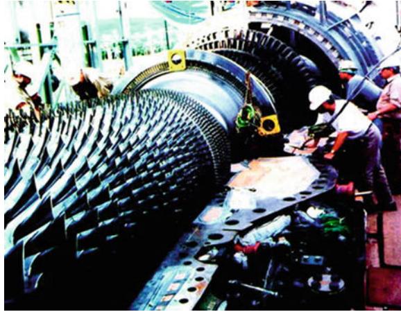
Fig. 2.4 Inspection of a steam turbine
